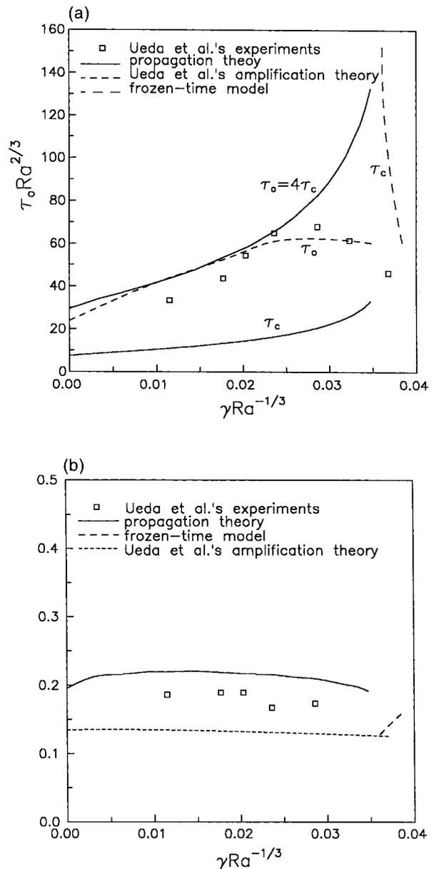
Fig. 3. Comparison of predictions (amplification theory with  $Pr = 8800$  and  $\dot{E} = 10^2$ ; propagation theory with  $Pr \rightarrow \infty$ ) at  $Ra = 15,000$  with experimental ones of  $Ra = 9000$ – $17,000$  and  $Pr = 8800$ : (a) characteristic times; and (b) associated critical wave numbers. Here  $\tau_c$  and  $\tau_0$  denote the characteristic time to mark the onset of convection and that of manifest convection, respectively.
