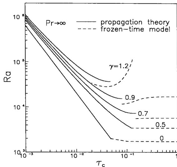
Fig. 2. Predictions of the critical time to mark the onset of convective motion.
